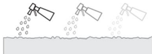
fig. 4.5: d) wetting the prepared surface
